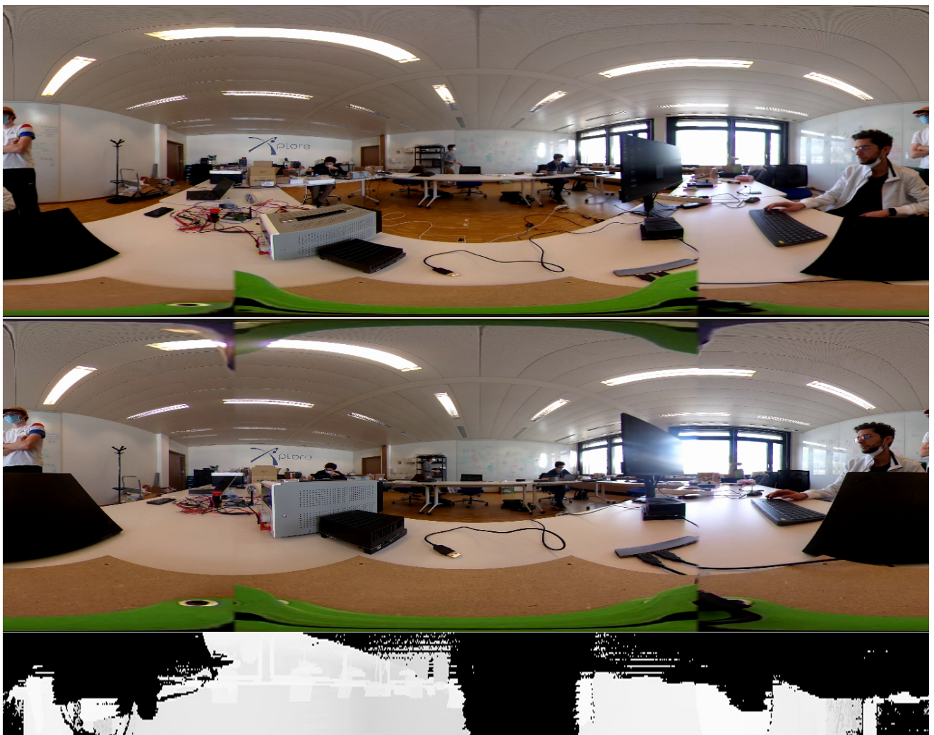
Figure 13: Upper camera /Lower camera / Depth map from the first dataset
